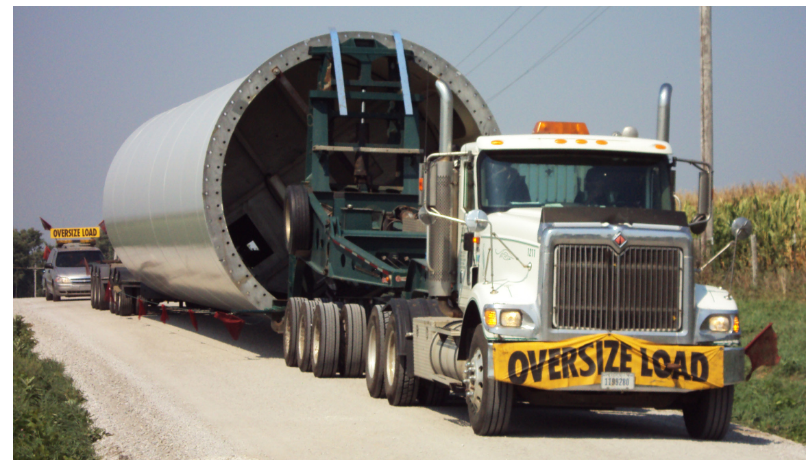
Step 4: Tower is Delivered in Sections
